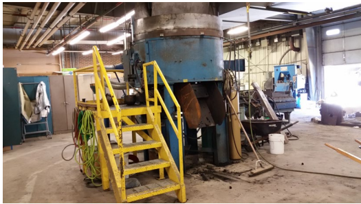
Figure 24. The green sand mixtures were produced using this muller.
