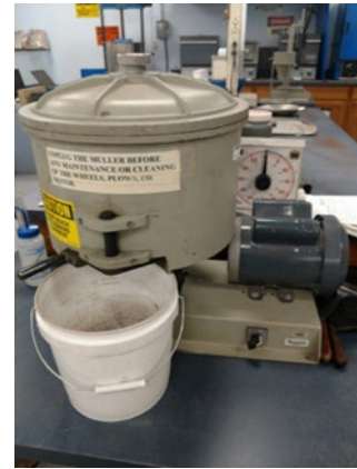
Figure 8. The prepared sand is muller in a laboratory muller.
