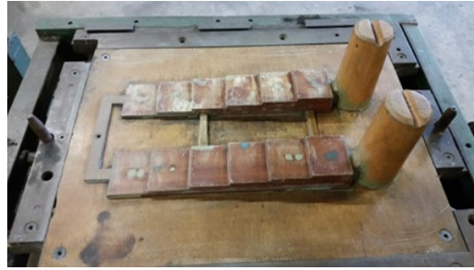
Figure 26. The step-block casting pattern (cope).
