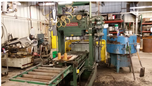
Figure 25. Molds were prepared using this molding machine.
