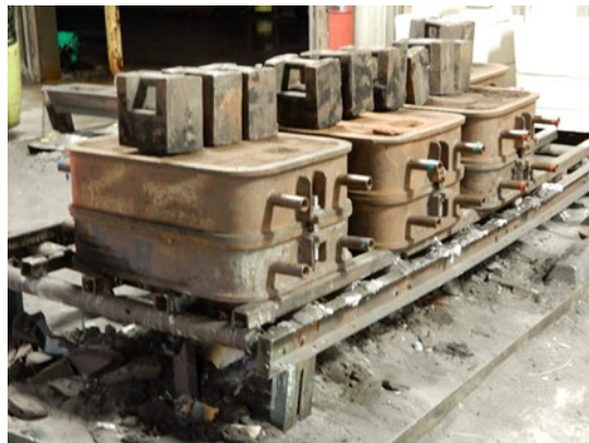
Figure 29. The prepared molds before pouring.
