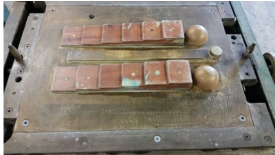
Figure 27. The step-block casting pattern (drag).
